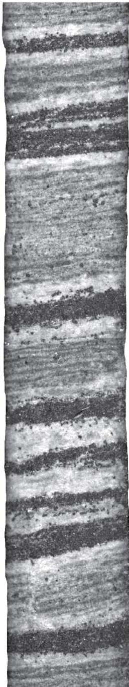
Figure 4: BIF drill core from the Kuruman Iron Formation, South Africa. Dark layers are composed of magnetite, light layers are siderite, and grey layers are composed of chert and hematite.
